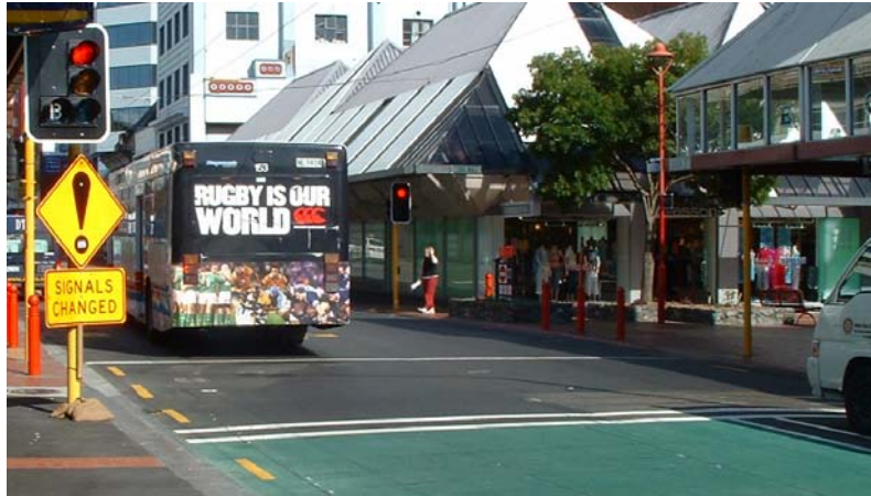
Signal pre-emption with priority lane on approach
